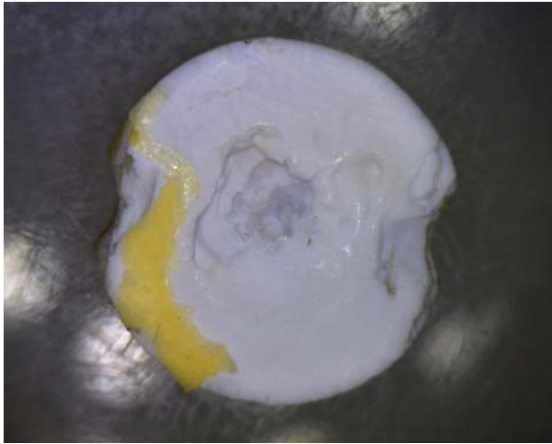
Fig. 2 – Image of the discoloration and dentin erosion on the loading surface of the specimen directly under the loading pin that occurred for type III experiments using the bleach sterilization method.
